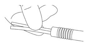
Push and connect the tubing securely and attach the handpiece handle over the cutting tip.
