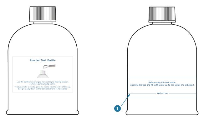
Before using this test bottle: unscrew the cap and fill with water up to the water line indicated. 1
