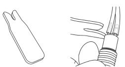
NOTE: Slide the key from the narrower tube side.
