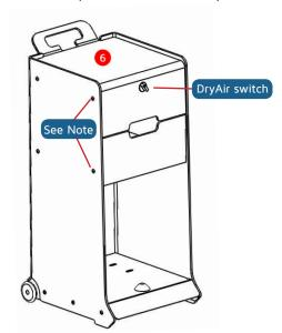
In order to position the top panel (#6). Slacken the front screws to the top and the drawer-support (as indicated above), enabling the top panel to be located into grooves.
